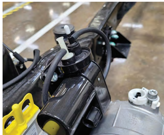
Cradle with Coolant Pump, AC Compressor, TXV Heat Exchanger, Vacuum Pump, and the Power Steering Pump
