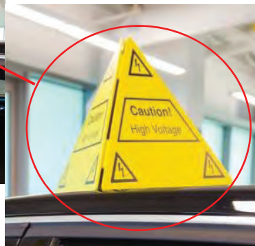
Marking of HV Vehicle in the Workshop
