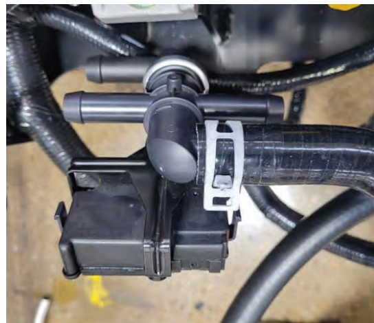
The 4-way valve is located on the back side of the center stack. The valve is controlled by the VCU "B".
