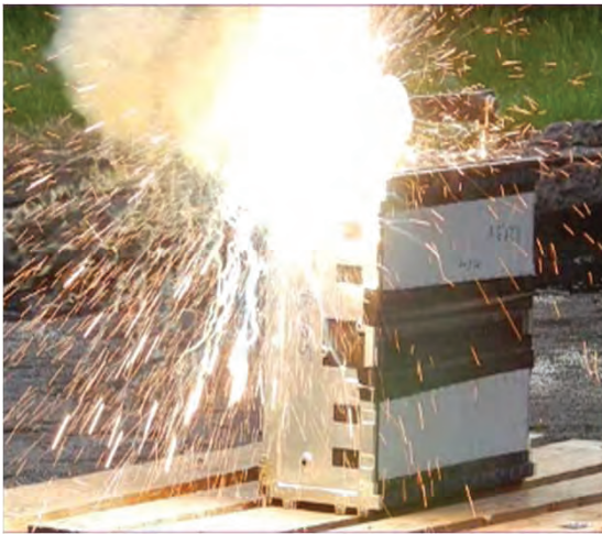
Electrical Arcs in HV Battery During Short Circuit Test
