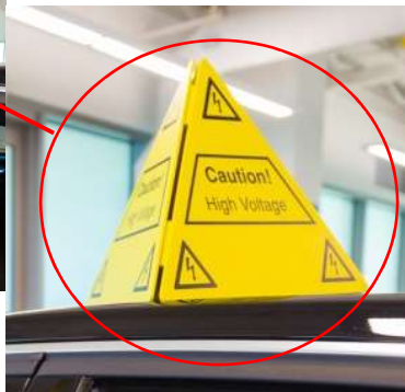
Marking of HV vehicle in workshop
