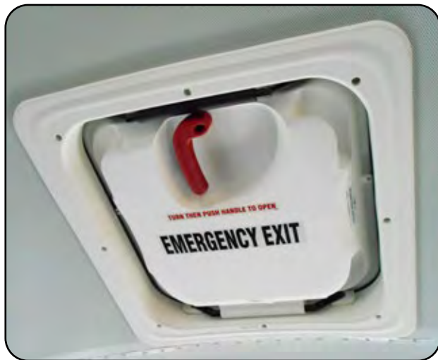
Figure 2-6 Emergency Roof Hatch
