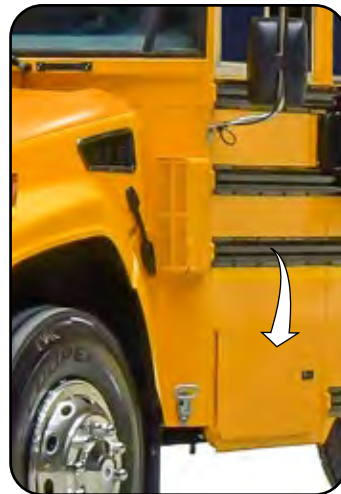
Figure 5-9. 12V Battery Box
