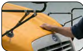
Pull forward lightly on the front handhold.
