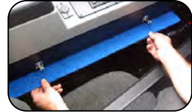
Figure 2-19. Heater Filter Access
