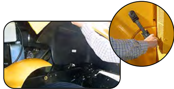
Gently lower the hood into position and re-latch the hold-down latches.
