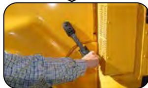
Release the hood hold-down latches.
