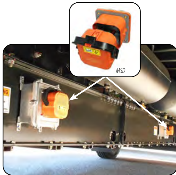
Figure 7-1. High Voltage MSDs (located on RH (curb side) under skirt)
