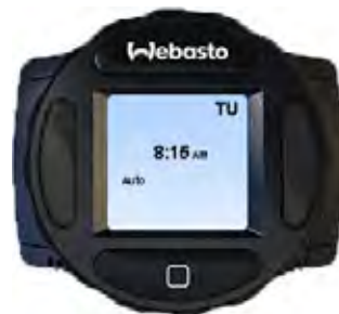
Figure 2-18. Webasto Digital Controller (located in the heater switch panel)
